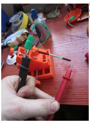
Finally, test the connections like you would our normal electrodes. You only need to lightly touch silver wire to test connection
