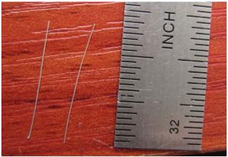
Cut % inch lengths of the silver wire, and burn off the ends with a lighter
