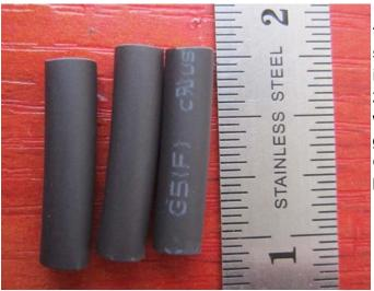
Cut three lengths of heat shrink tubing. Note this is smaller than our standard heat shrink tubing. This is .187 inch outer diameter (before shrinking) for 20-18 gauge, unlike the standard we use, which is .25 outer diameter, for 12-16 gauge. I have ordered some from Grainger, but you can get some from hardware store in interim
