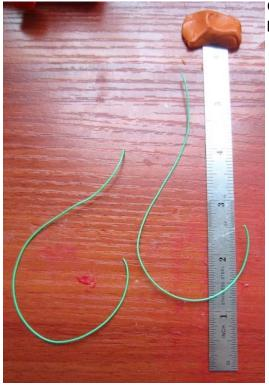
Cut two lengths of 7 inches of the green microwire (I left some with the RoboRoach supplies)
