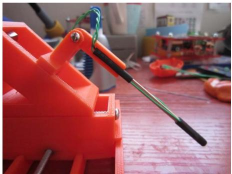
What's nice about this new design is that the heatshrink and wood can comply a bit so that the electrode fits inside with a friction fit (no silly putty needed)
