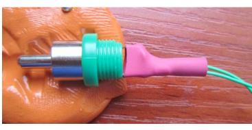
Put ¾ inch heat-shrink on, and glue and screw on cap like in our normal electrodes
