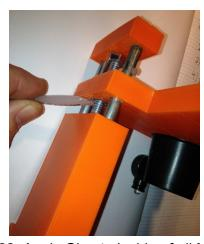
22. Apply Glue to inside of all Magnet Holes, and install Magnets.
