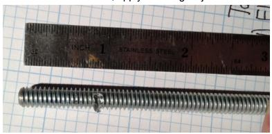
15. And Screw On Nut over glue so that nut ends at exactly one inch. Wait a couple minutes for glue to set.
