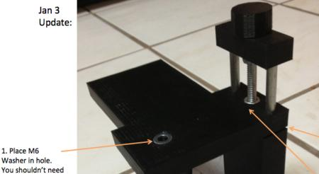
3. When shipping, Turn Knob and adjust height so that phone platform is almost touching microscope base piece. This is the "Default" configuration that works for most objects unless user puts an object >2 inches under scope
