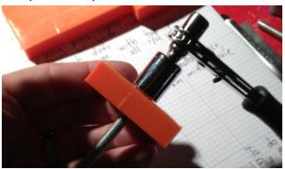
14. On the threaded rod, apply a bit of glue just before one inch mark....
