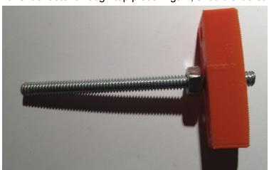
17. Apply a bit of glue to exposed top of bolt, and glue another nut. Make sure orange piece can turn freely between two nuts. Not too loose, not too tight. Then, slide knob on top of nut. Glue shouldn't be necessary as it's a friction fit. Use your discretion.
