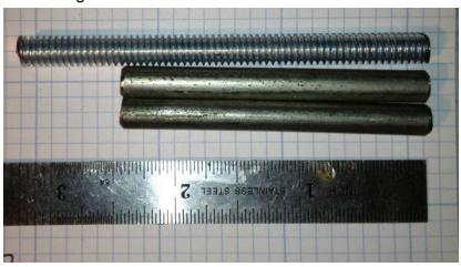
5. Lightly work smooth rods into side holes of bottom piece so that they slip in and out (going all ½ inch down) with some elbow grease. Don't excessively ream. You might find pliers useful.
