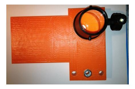
12. We have to ream middle hole of top piece so that the bolt turns easier withother gripping the plastic and hurting user's hands. Built a reaming tool by super-glueing a nut on the top of a spare threaded rod.
