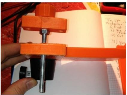
19. Put Guide Rods into bottom piece, again ensuring they go all ½ inch down. use glue at bottoms. Definitely add glue to tops...
