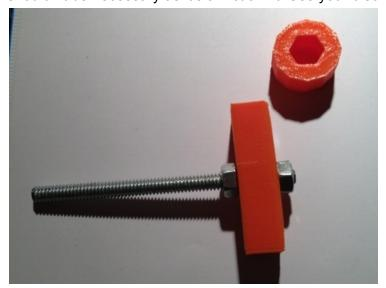
18. Screw Fastener through middle stage, leaving about a half-inch of clearance between sections.
