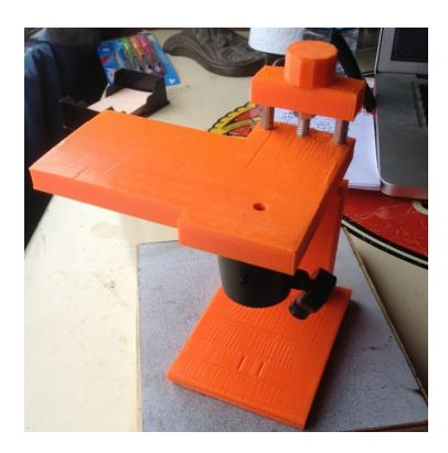
25. Make sure light turns on and check image quality. If image is distorted it means lens is not installed flatly or 3D print was not level and is at angle. Imaged below is 1x through iPhone and unzoomed. There should not be any plastic "shadows" around the edge of image. Plastic shadows can be caused by bits of plastic strands hanging out inside hole.
